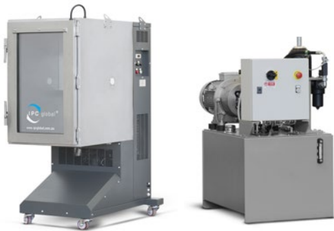
UTM-130 Environmental Chamber Hydraulic Power Supply
