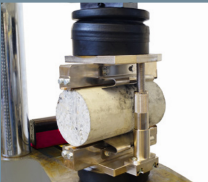
Splitting on concrete
