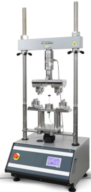
70-T1192 with accessories to perform flexure test on glass-fibre reinforced cement to EN 1170-5
