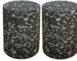
Up to two 150mm diameter cylindrical specimens for Texas Overlay Test
