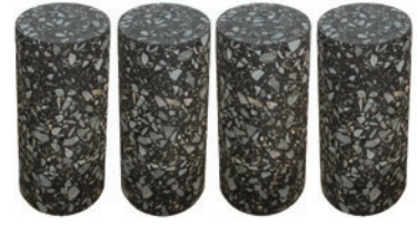
Up to four 100mm diameter cylindrical specimens
