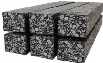
Up to six 50mm wide prismatic specimens
