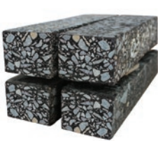
Up to four 70mm wide prismatic specimens
