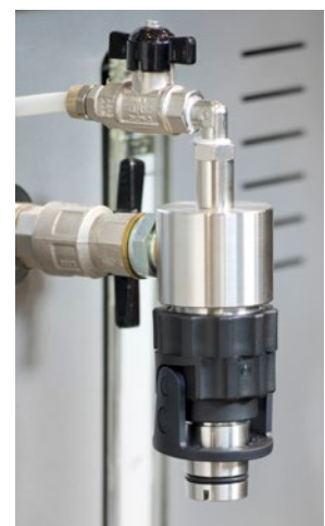
Detail of 75-PV5 X100 fast connection for Rotary evaporator flask, for bitumen solution sampling
