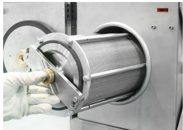
Placing the washing drum into the machine
