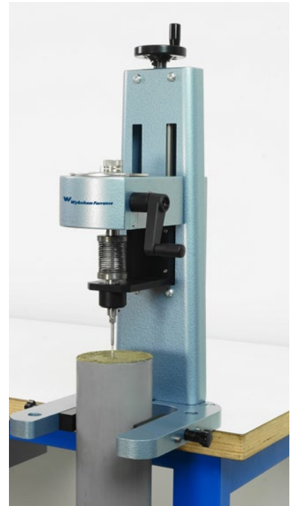
Vane Apparatus (27-WF17D30) fitted with holding sampling tube (27-WF1738) and 100 mm sampling tube.
