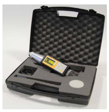
Rebound digital test hammer supplied complete with case (model 58-C0181/DGT)
