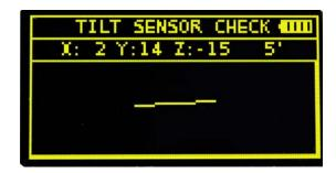
Example of digital hammer screen display - Measurement and indication of the exact instrument tilting angle by triaxial inclinometer
