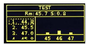
Example of digital hammer screen display – Test results displayed as numerical and graphical
