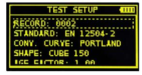
Example of digital hammer screen display - Test setup
