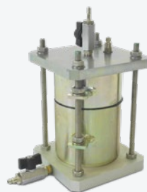
Falling Head Apparatus with compaction mold permeameter
