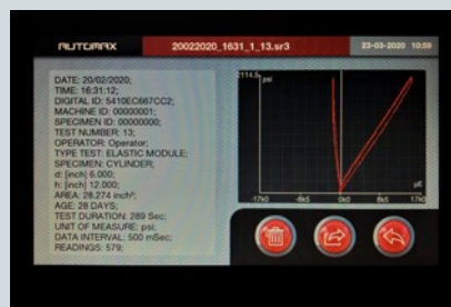
Elastic Modulus and Poisson ratio determinations
